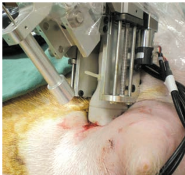
This robotic system is designed to help surgeons insert a radiofrequency ablation needle into a breast tumour as demonstrated on this goat.
